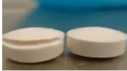
Gambar II. 4 kerusakan tablet capping
