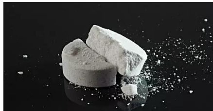
Gambar II. 5 kerusakan tablet splitting
