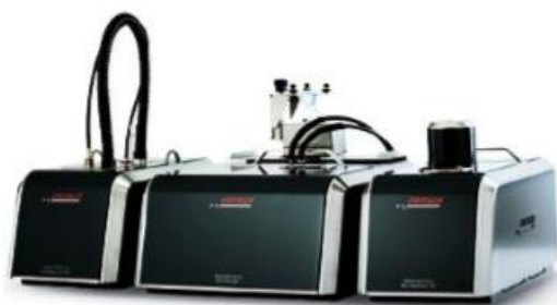
Gambar 2.8 Alat Particle Size Analyzer (PSA) Fritsch Analysette 22.
